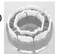
Picture 3 : Old motor is half assembly by manual whereas new motor is proceeded by machine and the cores are independently divided.
